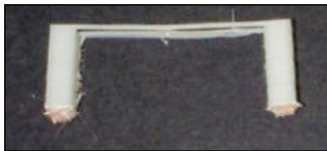
Figure 5. Bridge and cantilever geometries and results: (a) Initial bridge with increasing spans; (b) modified bridge with tall vertical columns; (c) cantilever.
